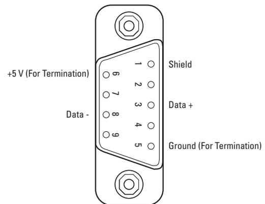
Figure 1. 9-Pin D-Sub Connector
