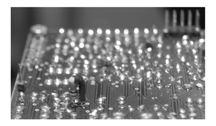
Here's what the resistor should look like when soldered to the pads of R54, again note the position compared to the reference holes.
