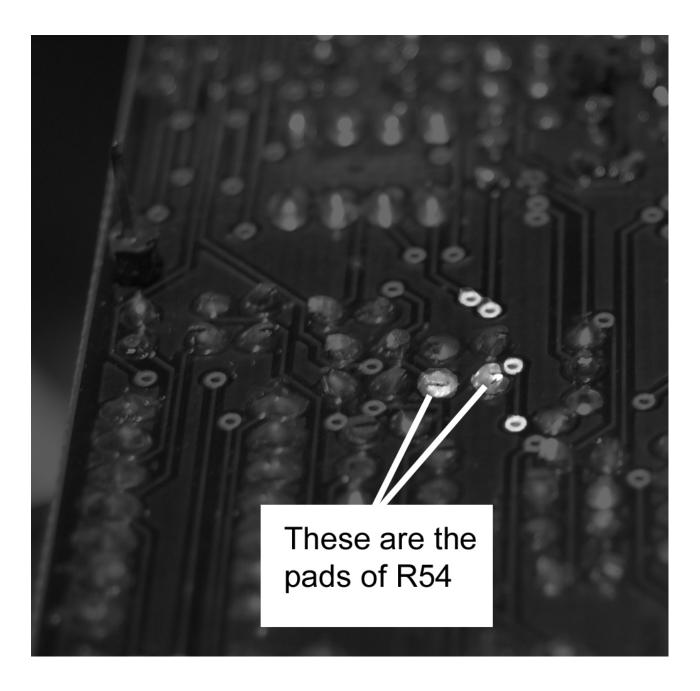
Here you can see the pads of R54, this is where you will solder the 10K resistor to. The four reference holes are highlighted to help you locate the position.
