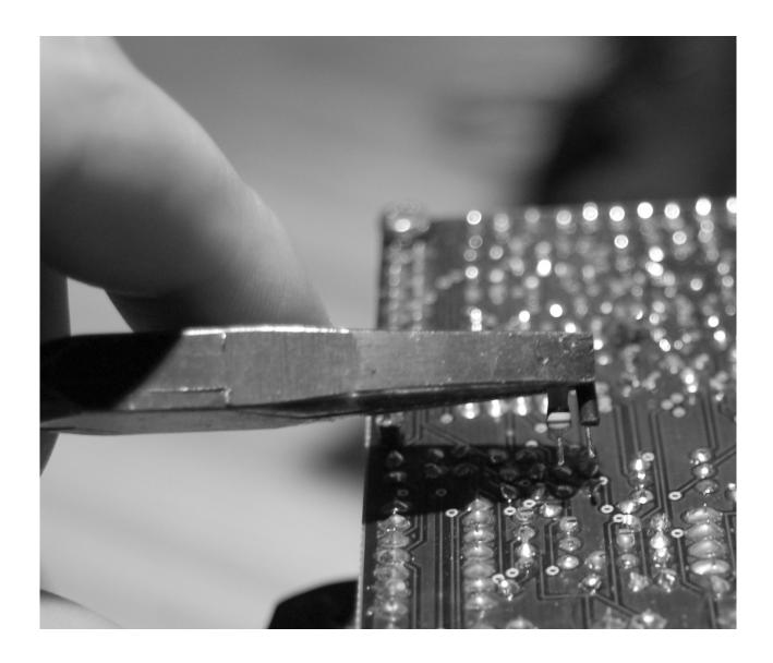
Use a pair of pliers to hold the resistor in place, I'm not holding the resistor on the pads in this photo, just slightly above them.
