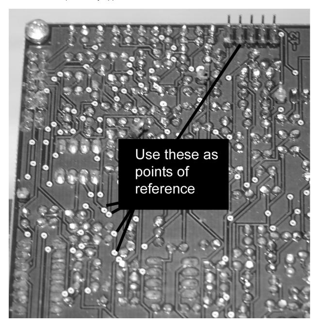
Disconnect your DrumDokta from your case and lay it face down on on a table with the power connector at the top. Use the above picture as a position reference.
