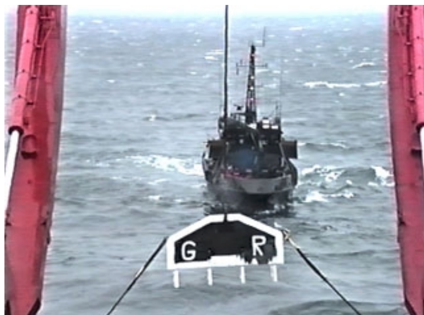
Picture 4. The picture shows the yoke hanging over the water at the first attempt to recover the visor. In the background, HMS Furusund.
