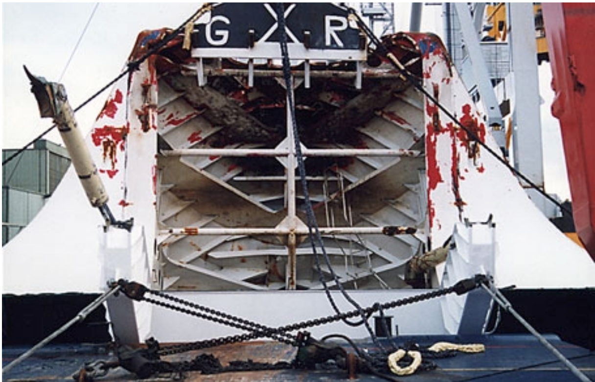
Picture 6. The yoke (marked G X R) hooked into the visor after recovery.
