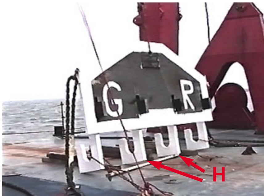
Picture 3. The picture shows the yoke hanging from the aft crane on the MSV Nordica. The four hooks can be seen hanging from the yoke (H).
