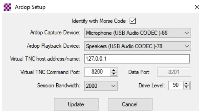
Search on the combo box for some *USB Codec* and select it for Capture device (*input to PC*) and Playback Device (*Output to Radio*)
