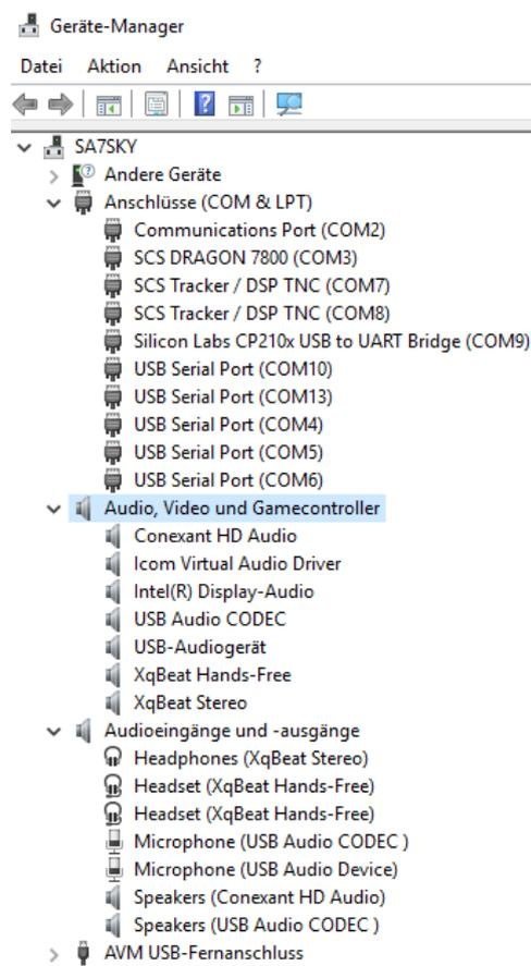
On the PC, the USB⇌COM is identified as *COM9*, essential for setting the Winlink. Check the USB Audio board.
