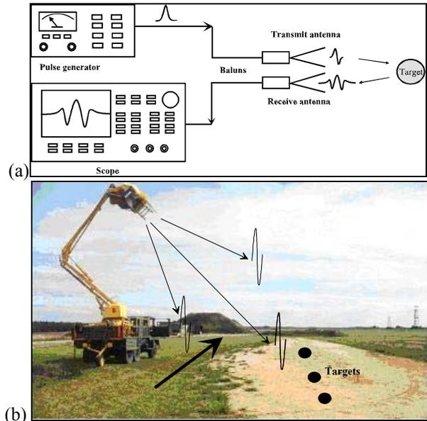
**Figure 1.** The UWB synthetic aperture Radar PULSAR
