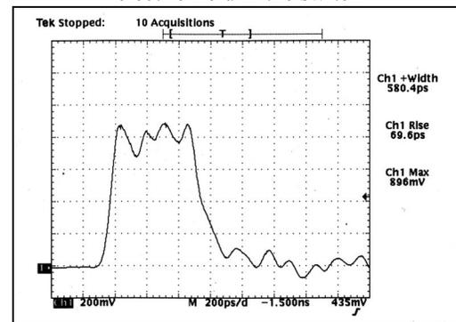
Figure 6. Output pulse shape of the coaxial generator (P=55bar, d=0.45mm, τ=68ps, V<sub>OUT</sub>=26kV)
