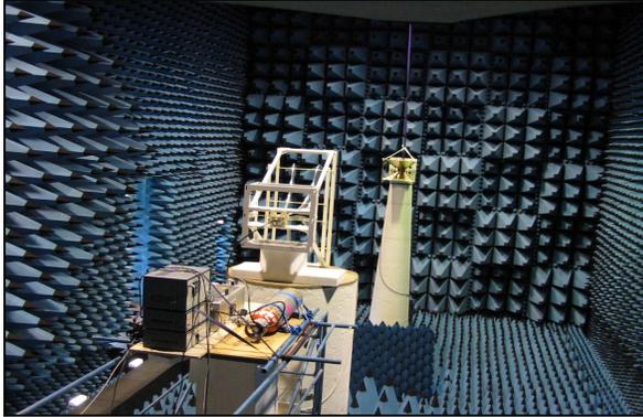
Figure 6. Characterisation test in an anechoic chamber
