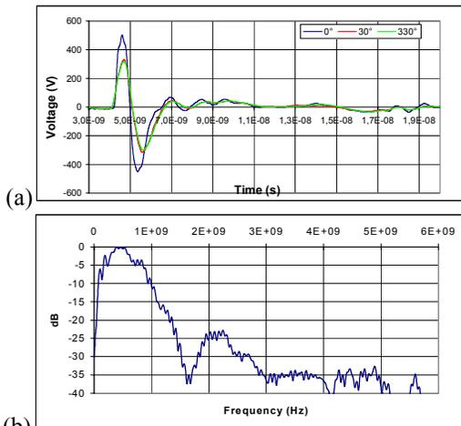
Figure 7. Measured signal at the receive antenna for antennas positioned facing each other (a) transient response (b) Fourier transform of the transient response
