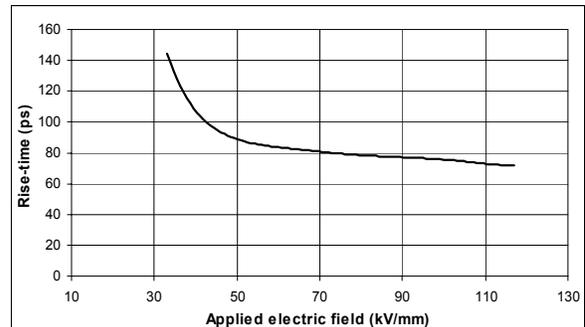
Figure 5. Rise-time of the output pulses versus electric field in the switch
