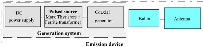
Figure 2. Basic structure of the pulsed power generation system
