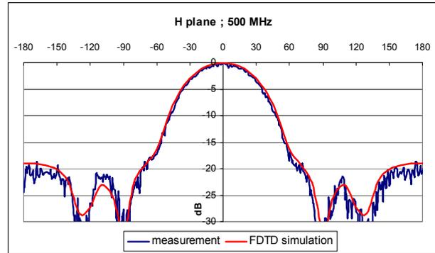
Figure 8. Radiation patterns in H plane (500MHz); transient measurement compared to FDTD method
