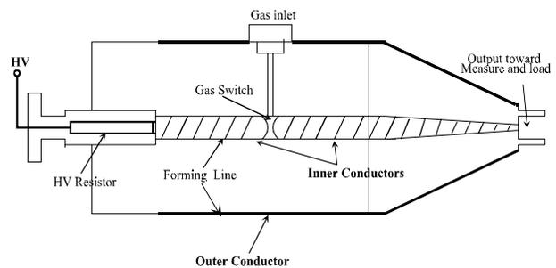
Figure 3. Schematic representation of the coaxial generator using a high pressure gas switch
